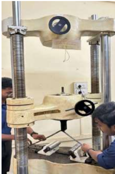
Fig.-5: Re-Bend Test on TMT bar
