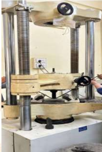
Fig.-4: Bending Test on TMT bar
