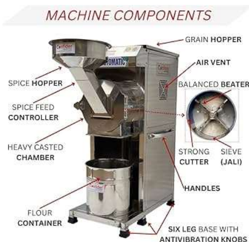
Fig -2, Showing Jamun seeds pufferizer machine
