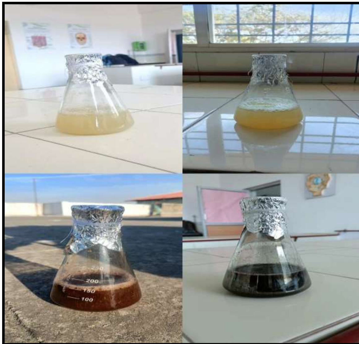
Fig 3 :- shows the periodic colour change of reaction mixture at different time intervals. (fenugreek seed extract+ 1mM AgNO 3 )
