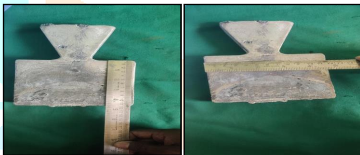
FIGURE: 5 CASTING IMAGE WITH DIMENSION
