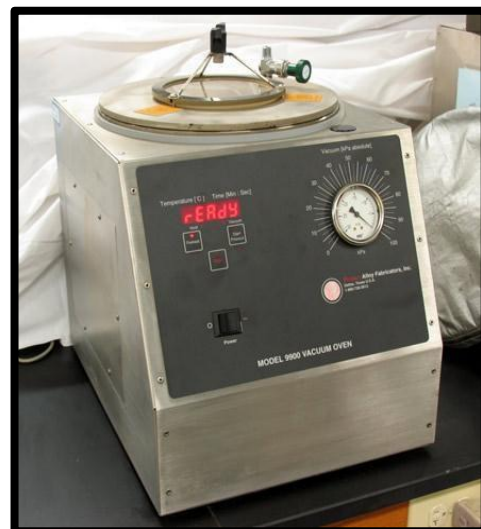
Figure 4: Vacuum Oven for degassing
