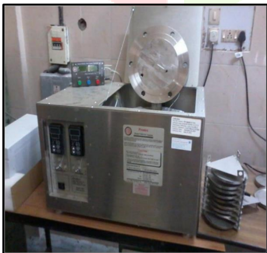
Figure 3: Pressure Vessel Aging for long term aging
