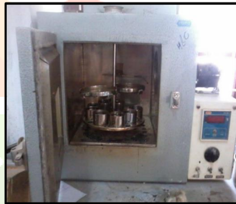
Figure 2: Thin Film Oven for short term aging
