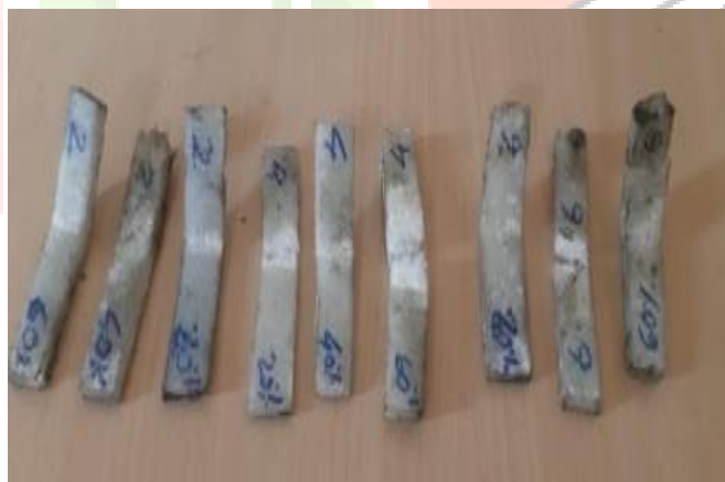
Figure 3. The specimens of composite material after impact test
