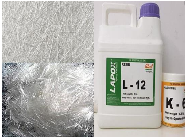
Fig.1:-Glass with Epoxy resin and K-6 hardener.
