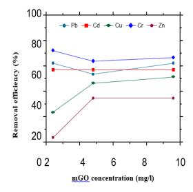
Although the removal efficiency of modified graphene oxide is not better than that of purchased graphene oxide, it is thought that the concentration of modified graphene oxide, which has the highest effect. removal has shifted to a lower concentration.
