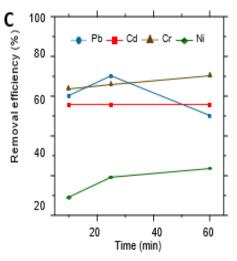
Above figures shows the influence of treatment time on the removal efficiency of purchased graphene oxide at the concentration of A, 2.4 mg/l, B, 4.8 mg/l, and C, 9.6 mg/l.
