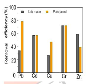
The **figure** shows a comparison of the removal efficiency of laboratory-produced graphene oxide and purchased graphene oxide.
