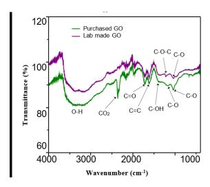
The reason for the difference in selectivity between purchased graphene oxide and laboratoryproduced graphene oxide is due to structural differences. Figure 12 shows the FTIR spectra of two graphene oxides [18].
