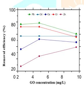
The figure shows the removal efficiency of labmade graphene oxide for various heavy metals. This indicates that graphene oxide has the highest Cr removal efficiency, which can reach 72.2%. Note that the Cr concentration after treatment was below the detection limit of the device, so the actual removal effect was higher than 72.2. The second highest removal efficiency is for Zn, and 59.4% of Zn in wastewater can be removed by graphene oxide.
