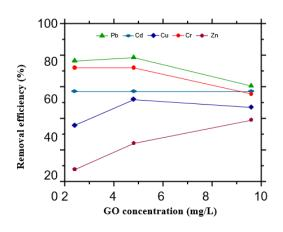
Unlike the laboratory-produced graphene oxide, the purchased graphene oxide has a high removal effect on Pb, reaching 78.6% at a graphene oxide concentration of 4.8 mg/L.
