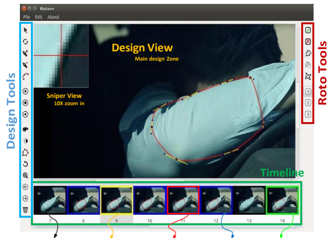
Figure 4: A screenshot of our interactive tool Roto++. This user interface consists of a design view, design tools, roto tools and a timeline. This timeline encodes our frame selection feedback by using colored borders. A full user guide to our tool is included in the supplemental material
