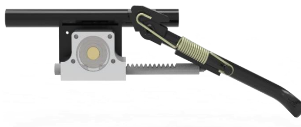
Fig -12: Automatic system pushing the side stand.
