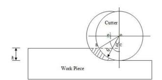
Fig. 3. Chip Cross Section
