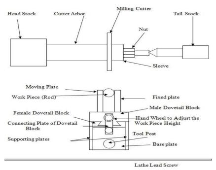
Fig. 4. Top view of slotting and milling attachment to lathe
