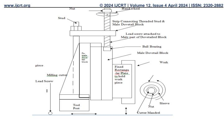
Fig. 5. Right side view of slotting and milling attachmentto lathe
