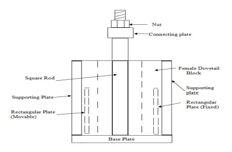
Fig. 6. Front view (operator side) of slotting and millingattachment to lathe
