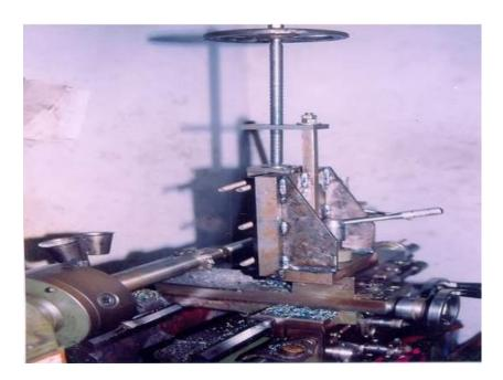
Fig. 1. Isometric view of entire attachment
