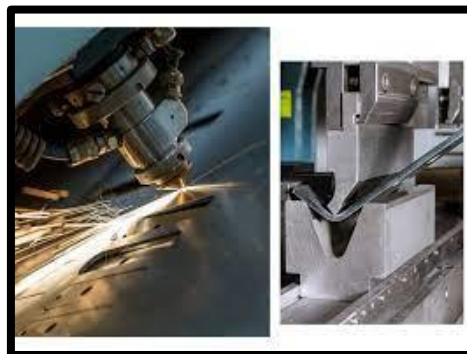
FIG.1.11 Aluminum Sheet - Laser Cutting Technology - Bending Process
