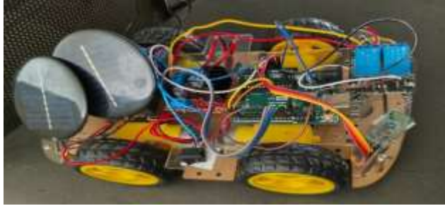
Fig.2: Outcome of Solar based Grass Cutter
