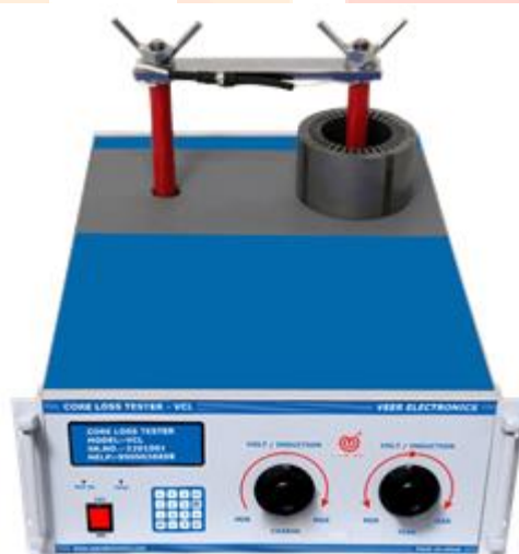
Figure 12: Core Loss Tester (Courtesy: Veer Electronics)
