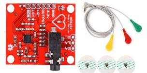
Figure 2: AD8232 ECG Sensor
