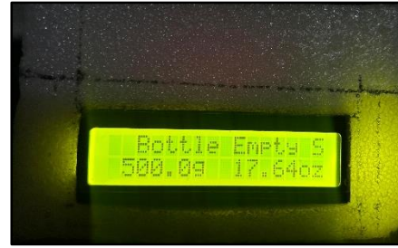
Fig 5.6: Displaying weight when IV bottle connected
