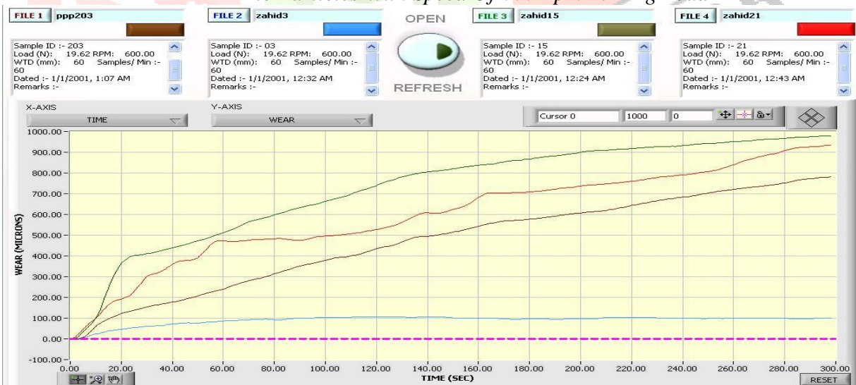
Fig 3.10: Comparison of Wear Behaviour Graph Of Al-7068 Composite Reinforced With 0, 3, 9 & 12% Tic Particles With Speed Of 600 Rpm At 2 Kg Load
