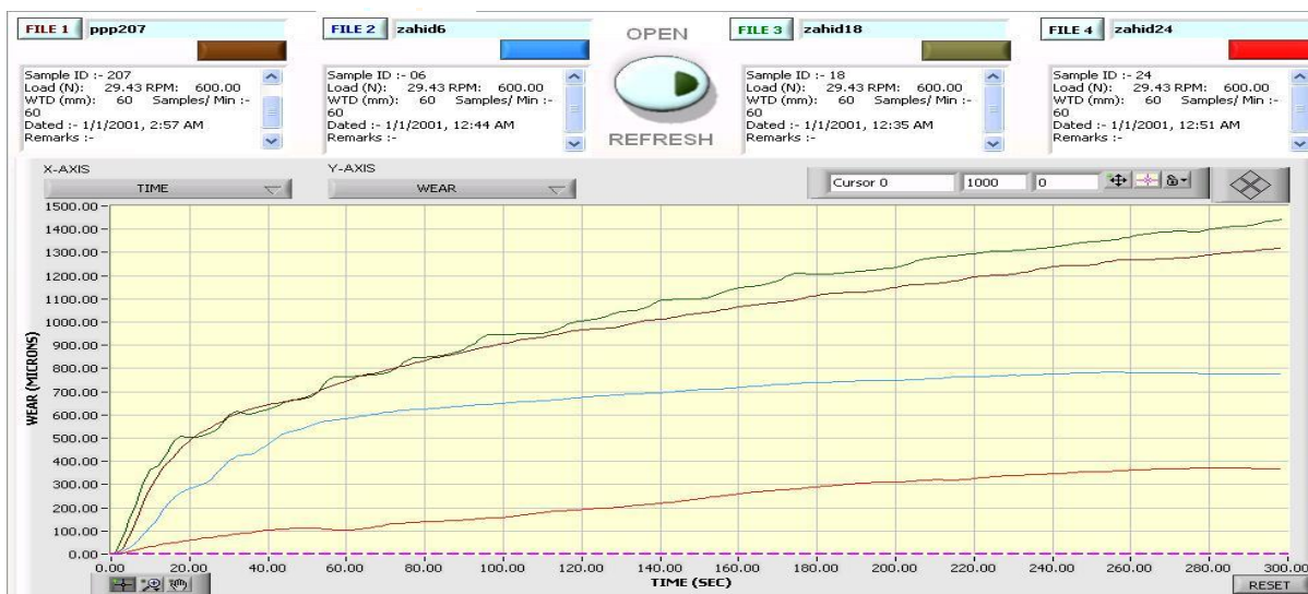
Fig 3.12: Comparison of Wear Behaviour Graph Of Al-7068 Composite Reinforced With 0, 3, 9 & 12% TiC Particles With Speed Of 600 Rpm At 3 Kg Load
