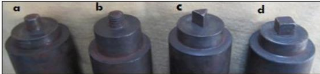
Fig.1.2 : different pin profiles; (a) Straight cylindrical. (b) Threaded. (c) Triangular (d) Square
