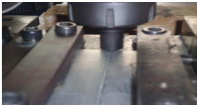
Fig.1.3.Experimental setup for FSW
