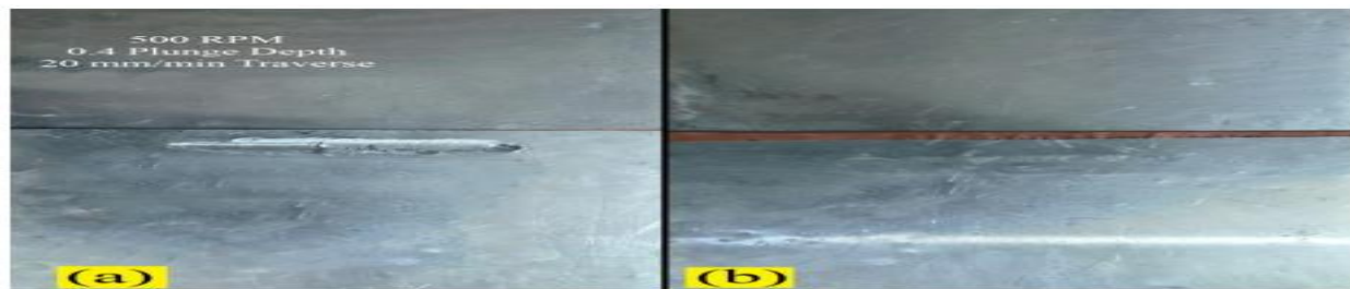
Figure.2.3: 500 RPM; 0.4 mm Plunge Depth; 20 mm/min Traverse Speed (a) Front Side of Weld (b) Back Side Of Weld
