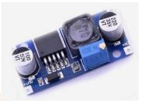
Fig. buck boost converter
