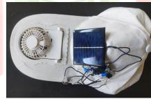
Fig. Solar cap with mobile charging
