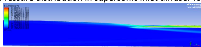
Fig.22:Pressure distribution in supersonic inlet diffuser for case-19
