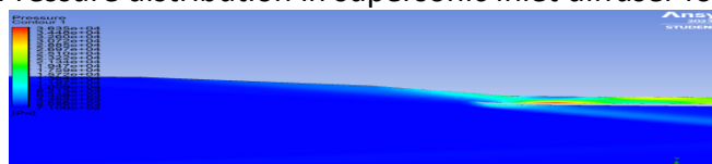
Fig.23:Pressure distribution in supersonic inlet diffuser for case-20
