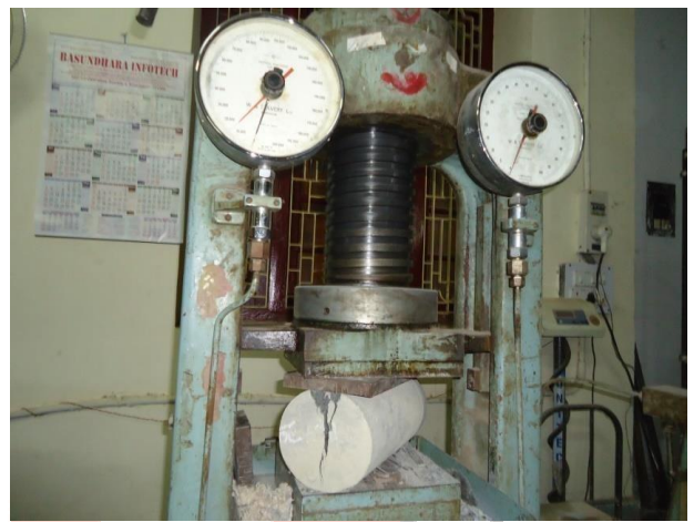
Fig: 3.2.6.2 Split tensile Test Set-up
