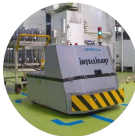
Fig 3.1 Line Following AGV
