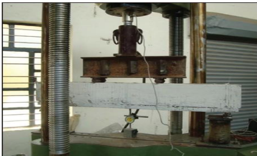
Figure 8.2 : UTM Test on Strengthened Beam
