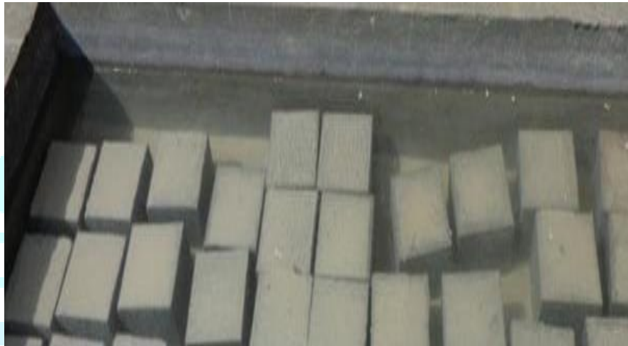
Figure 6.2 Cubes left for curing
