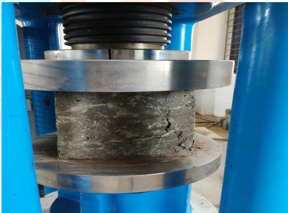
Figure 6.4 Compressive Stress acting on cubes
