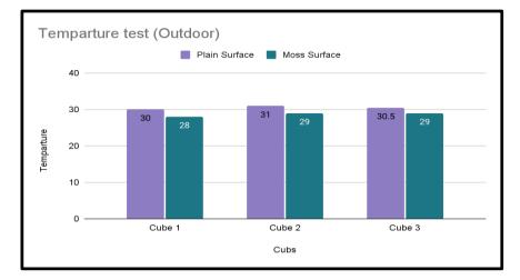
The temperature of concrete cubes ranges from 1°C to 1.5°C. Growing moss on large areas such as walls, roofs, and facades can reduce temperatures by 4°C-5°C, contributing to green buildings and sustainable construction. The urban heat island effect, which is a big issue nowadays, can also be minimised using this. And the use of air conditioners will be minimised. So, the use of these moss-grown walls should be promoted.
