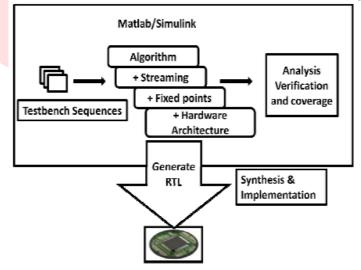
Fig.3. Workflow for FPGA using MATLAB and Simulink
