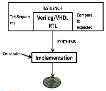
Fig.2. Workflow for FPGA using RTL/HDL
