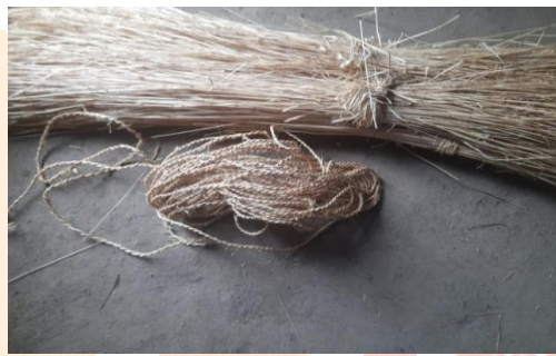
Fig 2. Hemp stalk and yarn twisted from it
