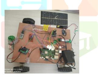
Figure 2: Prototype model of our Robot grass cutter
