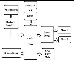
Figure 1: Schematic diagram of the Robotic Solar Grass Cutter
