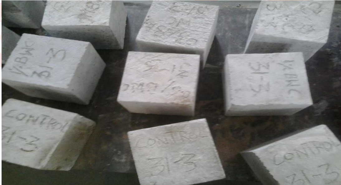
Fig. 3.3 (a): concrete cubes casted in the mould
