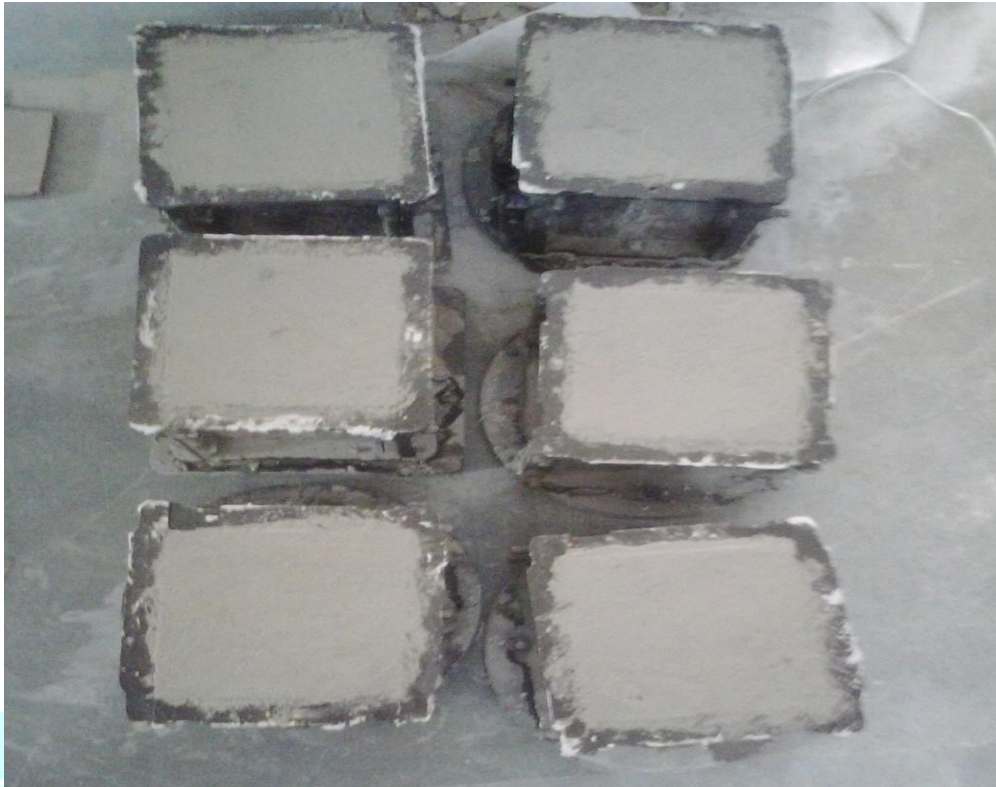
Fig. 3.3 shows some concrete specimen casted in laboratory
