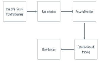
The proposed system is a cost-effective real-time eye-tracking and blink detection solution using only a frontal camera. With four main components, it enables seamless eye-based cursor control and clicking, while also enhancing user engagement and driving safety through an alarm alert mechanism triggered by detected eye blinks.
