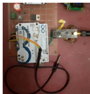
Audio Transmitter circuit
