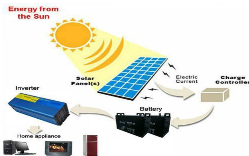
Fig. 2.1.1 Working of a solar energy system
