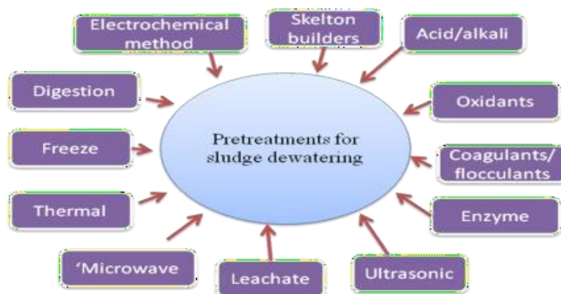
Fig. 2. Sludge dewatering of conditioning methods
