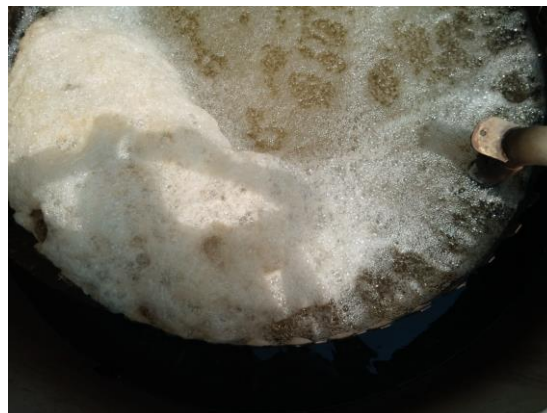
Photo 5: Image of Granular Sludge during aeration phase (Courtesy M/s Shreyans Energy P Ltd)
