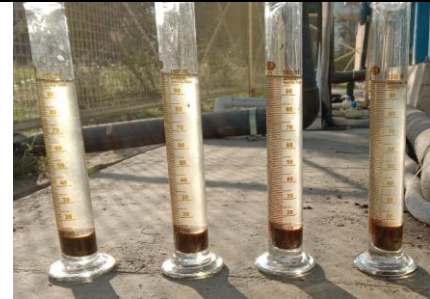
Photo 6: Sludge settlement with respect to time (Courtesy M/s Shreyans Energy P Ltd)
