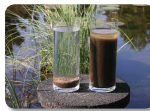
SVI comparison of aerobic granular sludge (left) and conventional activated sludge (right)
