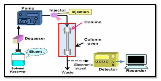
FIG.1.3Instrumentation high pressure liquid chromatography
