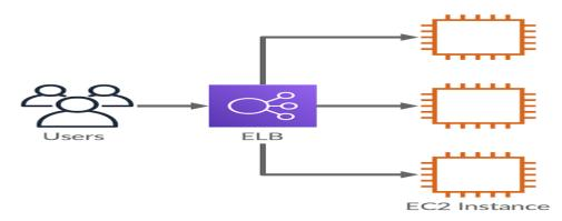
Figure 3.3 Traffic Distribution To Multiple Instance
