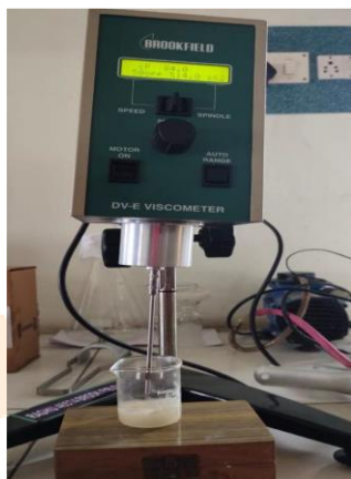
Figure 1: measurement of viscosity using Brookfield viscometer
