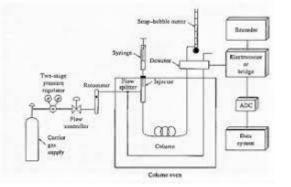
"Fig: -1" Schematic diagram of gas chromatography
