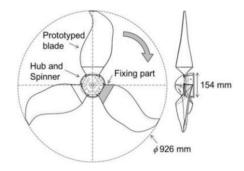
Fig.4. Biomimetic Wind Turbine
