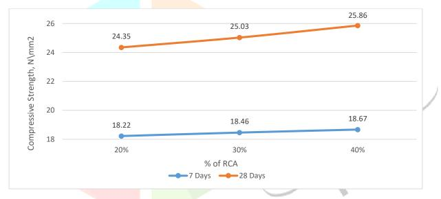
Compressive Strength for Replacement of NCA with 15yrs RCA and replacement of Fine aggregate with Silica Fume
