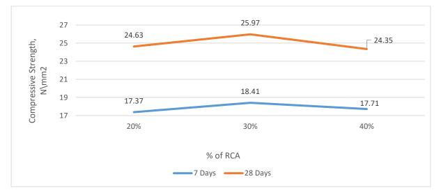
Compressive Strength for Replacement of NCA with 25yrs RCA and replacement of Fine aggregate with Silica Fume
