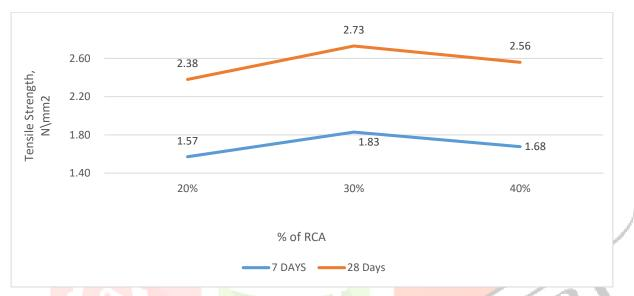
Tensile Strength for Replacement of NCA with 25 years and replacement of Fine aggregate with Silica Fume
