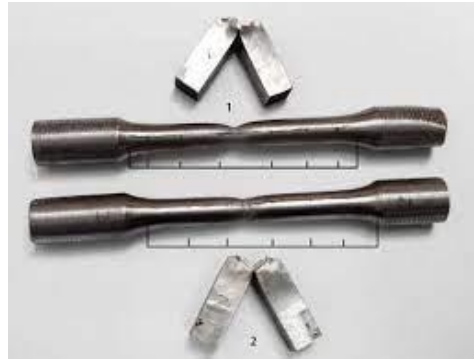
Figure 2: steel test – piece
