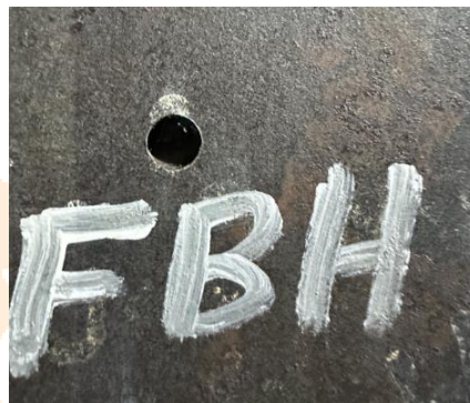
Figure 2A: Flat bottom hole test piece
