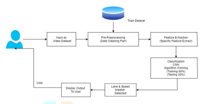
A system architecture for a lane and speed breaker warning system for vehicles using video input typically involves several components and stages:
