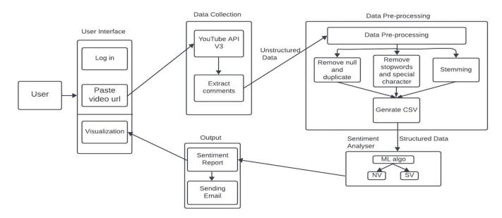
figure 1. Block diagram of a sentiment analysis system for YouTube comments
