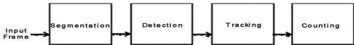
Fig.2.1 Overview of vehicle detection and counting system
