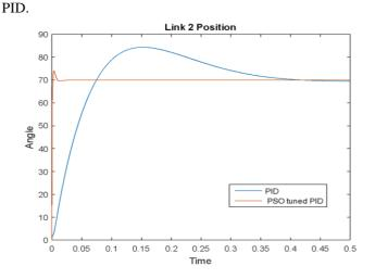
It is inferred that for link 2 the Settling time and the Rise time of PSO tuned PID is less compared to conventional PID. Hence the performance of PSO-PID is better when compared to conventional PID.
