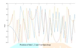
In Open loop, the control action from the controller is independent of the "process output". Since it is an open loop, the links will be moving in a random manner and there would be no control over the links. Therefore, we move to PID controller for Robot manipulator.
