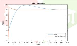
It is inferred that for link 1 the Settling time of PSO-PID is less compared to the conventional PID and also the Rise time of PSO tuned PID is less compared to conventional
