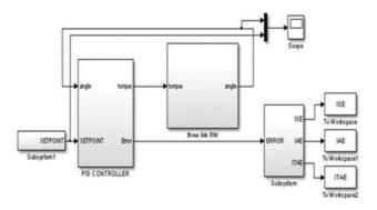
The PSO-PID is better when compared to Conventional PID in the Integral square error, Integral absolute error and Integral time absolute error analysis.
