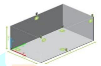
TDoA 3 mod has many similarities with TDoA 2 and supports all characters or Crazyflies. The main difference is that the slotting concept in TDoA 2 is replaced by transmission time, which makes it possible to add more anchors. By adding ports, the system can be expanded to a larger area or multiple rooms without having to find lines at each port. It also makes it stronger and can control the loss or addition of ports
