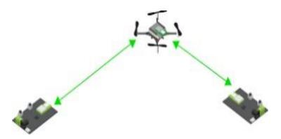
This mode is the most accurate and works even when the tag or Crazyflie is out of station. Active tags communicate with anchors in a time-slotted manner. Only one Crazyflie can be placed in this mode and a maximum of 8 anchors can be placed. In TDoA 2 mode, it continues to send packets parallel to the anchor.
