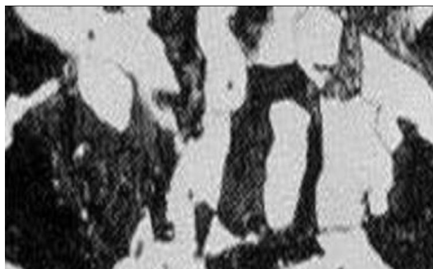
Figure 2.1: Microstructure of 1025 Steel Bar [23]
