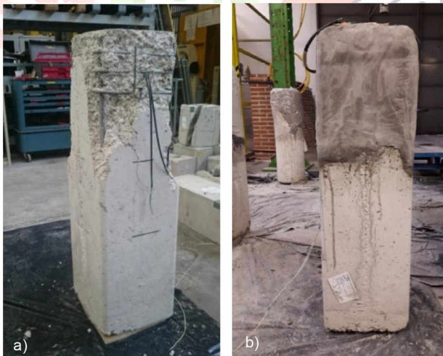
Fig. 3. S33_NC specimen after failure (a); S33_NC specimen after repair operation ( b ).
