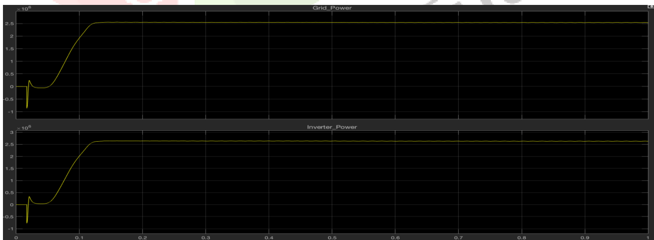
Fig. 15. Real Power at Grid & Inverter
