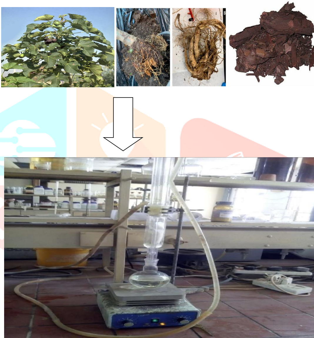
FIG:- 5 J.CURCAS ROOT EXTRACTION BY SOXHLET
