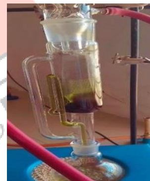
Fig.3- Soxhlet extractor for Leucas aspera
